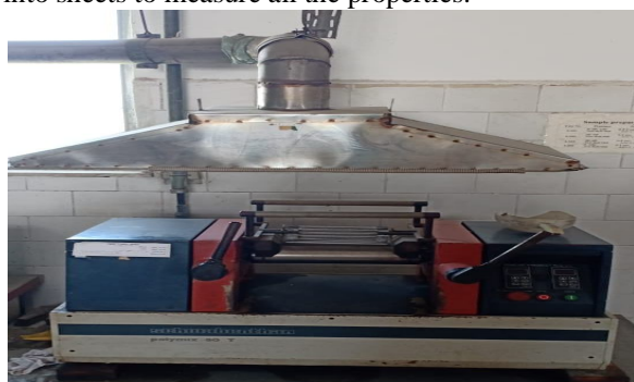
Figure (1): Two Roll Mill Machine
