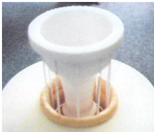
Fig.20 Cage being installed into a bag.
