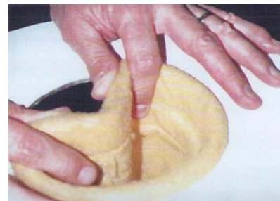
Fig.17 installing the bag into the tube sheet.
