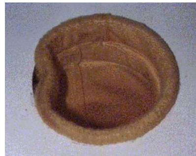
Fig.18 Incorrectly installed bag.
